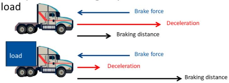
Brake force is identical, unaffected by initial speed and load!
